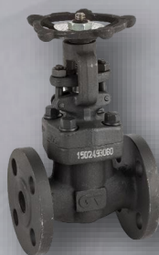
Schuifafsluiter, geflensd, ANSI 150 A105/N Gate valve, flanged ends, ANSI 150 A105/N
